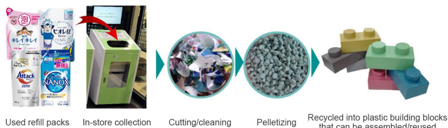
The process of recycling used refill packs in the RecyCreation initiative
